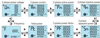
(note: in 3 phase 3 wire status only dislay 3 phase line voltage, current, total active power, reactive power, total power factor, frequency)
